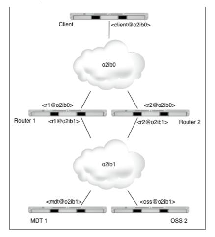
The NID's in the above diagram are represented symbolically (i.e. <r1@o2ib0>). The assumption is the test will be run on IB networks
