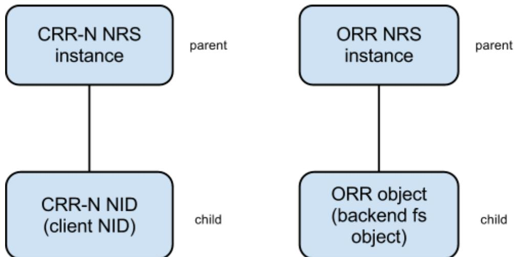
**NRS heads** (`ptlrpc_nrs`) act as containers of policy instances that are compatible with a given PTLRPC service. Each PTLRPC service has at least one NRS head for policy instances that are used for handling regular priority requests, and optionally a second NRS head for policy instances handling high priority requests (if there is provision in the given PTLRPC service for handling high priority requests).
