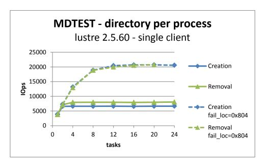
The plain lines show the file creation and removal rates on a single client in function of the number of tasks. The operation rates reach their maximum as soon as 4 tasks are running in parallel. This is because the Lustre client only allows one creation or removal request in flight at a time.
